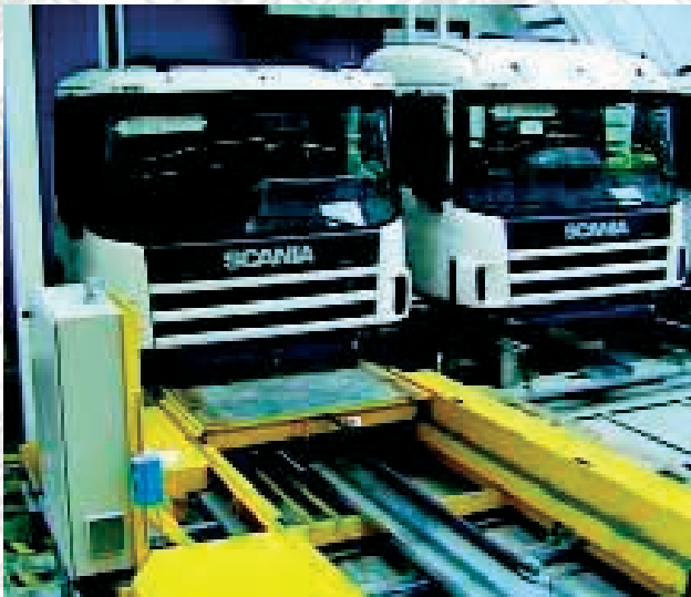
UNIVEYOR Shuttle Storage used as flexible buffer storage for cabins. From storage the cabin is delivered for overlift to on-line assembly.
